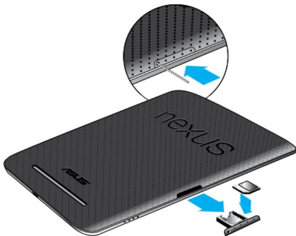
When the tablet is face down, the SIM card tray is located on the right side. The eject button is a small round opening on the left side of the tray door.
